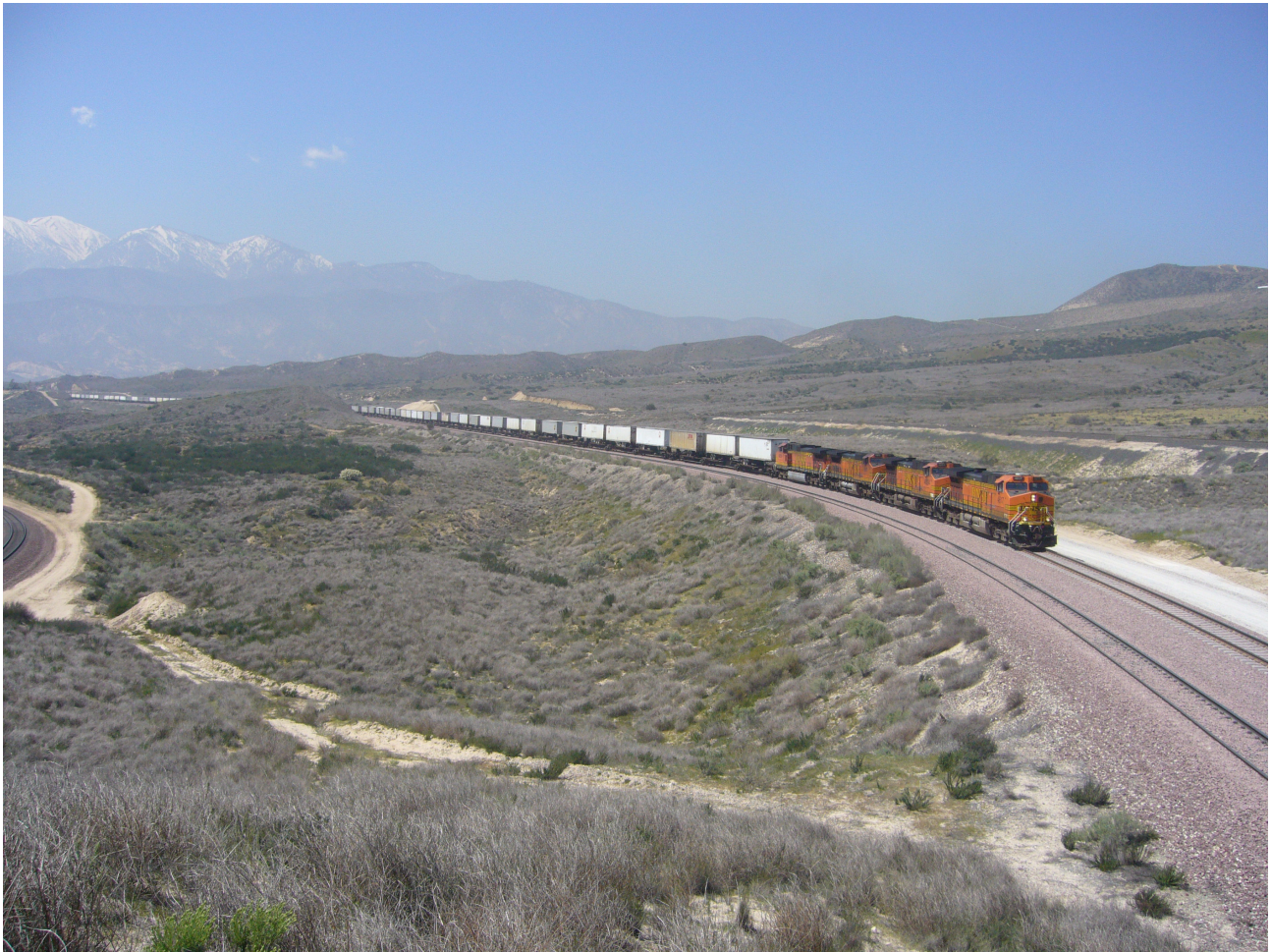
BNSF Extra 4817 East climbs Cajon on the new track about a mile west of Power Line Road with a mixed UPS/J.B.Hunt TOFC consist. Just visible on the far left side of the photo is the 1889 alignment track used primarily for downhill traffic due to its almost 3% grade. Visible to the right and a little above the BNSF train is the UP Colton Cutoff line.
