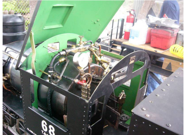
The cab sports a new reflex water glass
