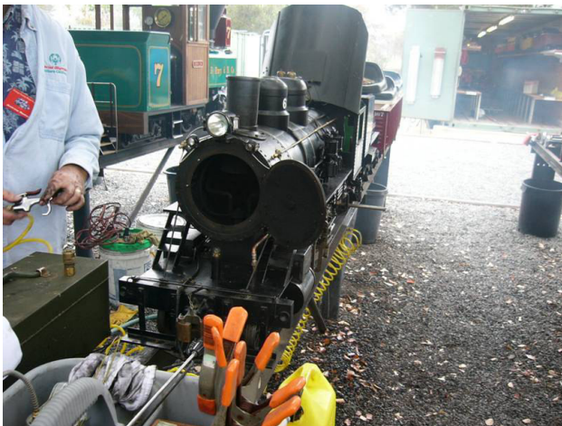
Here Andy gets ready to blow compressed air on "Emma" to rid her of soot, then he'll close the smoke box
