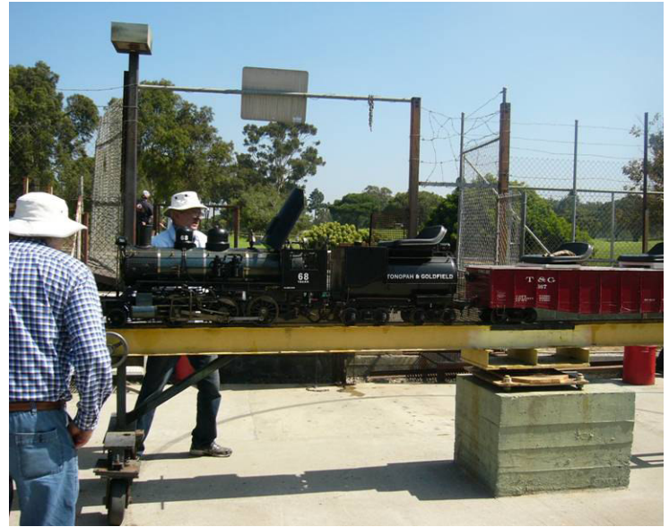
...and onto the transfer table to be returned to the steaming bay to be blown down, drained, cooled and cleaned.
