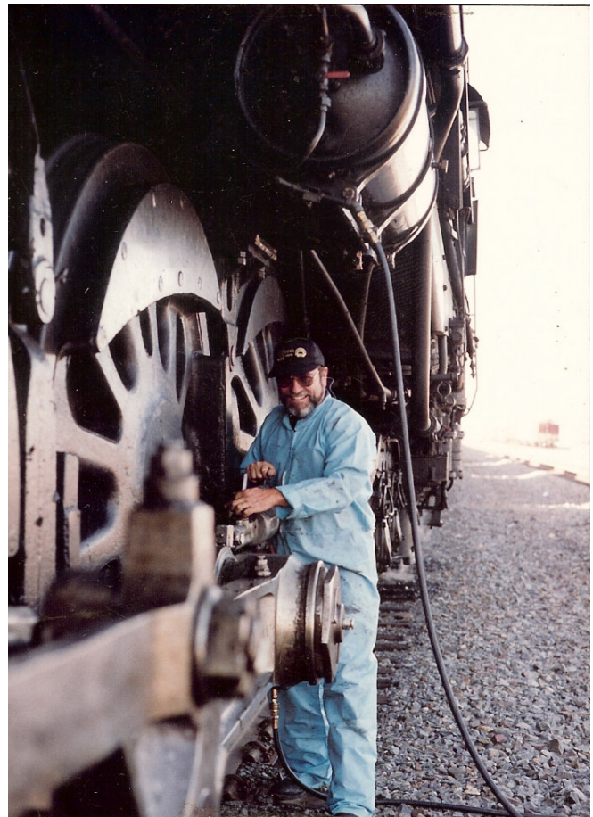
George Barlow uses a power greaser on the rod bushings, where they attach to the 7-foot-high wheels on Santa Fe No. 3751
