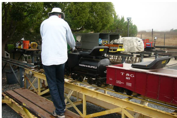
Now she has a full head of steam and is rolled from the steaming bay track onto the transfer table
